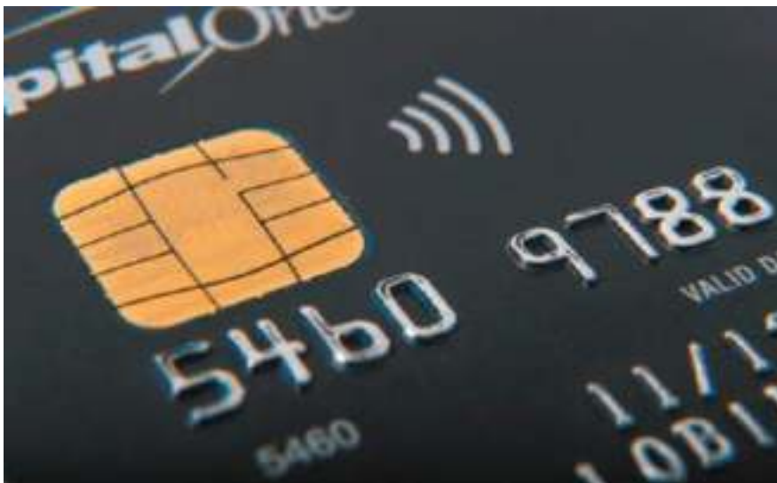
Smart debit or credit cards contain a microchip and are much more secure from fraud than are cards that only have a magnetic strip.
