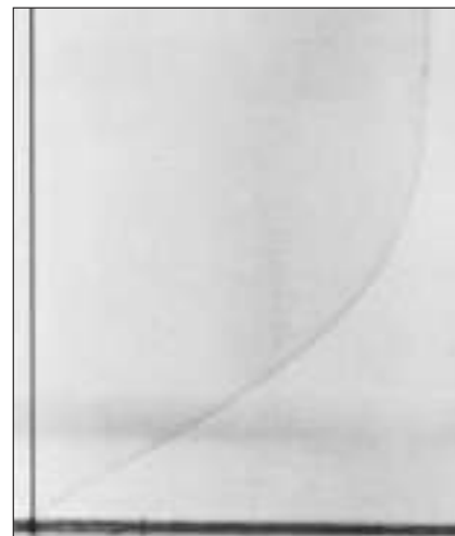
FIGURE 10-78 Flow visualization of a laminar flat plate boundary layer profile. Photograph taken by F. X. Wortmann in 1953 as visualized with the tellurium method. Flow is from left to right, and the leading edge of the flat plate is far to the left of the field of view. Wortmann, F. X. 1977 AGARD Conf. Proc. no. 224, paper 12.
