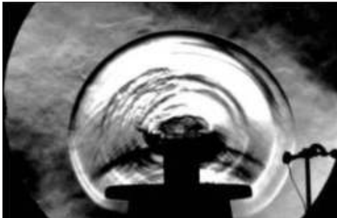
FIGURE 12-33 Schlieren image of the blast wave (expanding spherical normal shock) produced by the explosion of a firecracker detonated inside a metal can that sat on a stool. The shock expanded radially outward in all directions at a supersonic speed that decreased with radius from the center of the explosion. The microphone at the lower right sensed the sudden change in pressure of the passing shock wave and triggered the microsecond flashlamp that exposed the photograph. Photo by G. S. Settles, Penn State University. Used by permission.
