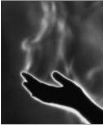
FIGURE 2-8 Natural convection over a woman's hand. G. S. Settles, Gas Dynamics Lab, Penn State University. Used by permission.
