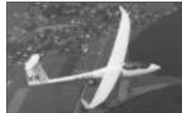
(b) Winglets are used on this sailplane to reduce induced drag.
